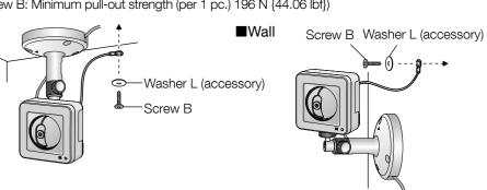
Wiring through a hole made in the ceiling or wall
