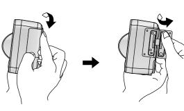
Insert the SD memory card with the label facing the rear of the camera and the pins facing the front of the camera. Gently push the card with your finger until it clicks.
